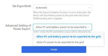
When allow PV and battery power to be exported to the grid, the PV and battery power will be allowed to be fed into the grid to obtain benefits at the same time.
