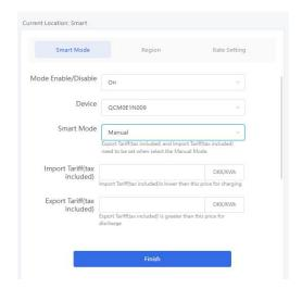
When the Smart Mode is enabled, the system will charge during low electricity price periods, discharge during high electricity price periods, and keep in Load First Mode during other periods.
